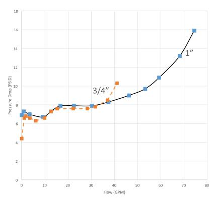
Meter Rated Flow as determined by approval agencies, 7.5 ft/sec is the typical maximum Plumbing system flow rate.
